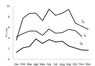
Fig. 1: Month wise percentage boiler losses  $(L_1, L_2 \text{ and } L_3)$
