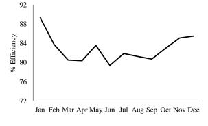
Fig. 2: Month wise percentage boiler efficiency
